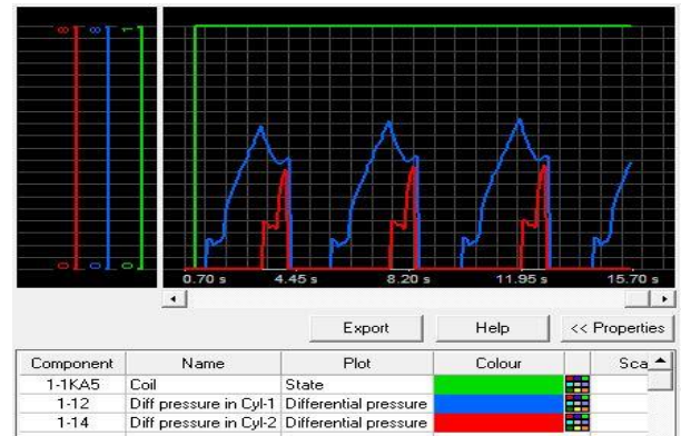
Fig. 8: Input vs. differential pressure of two cylinders
