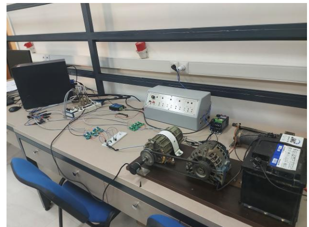
Fig 1_ Experimental platform of the electric drive and measurement system
