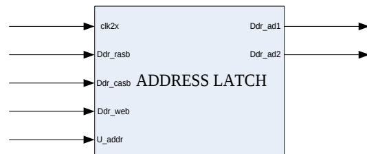
Fig. 5: Address latch module pin diagram
