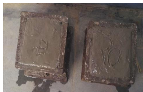
Fig. 3: Cubes after compaction.
