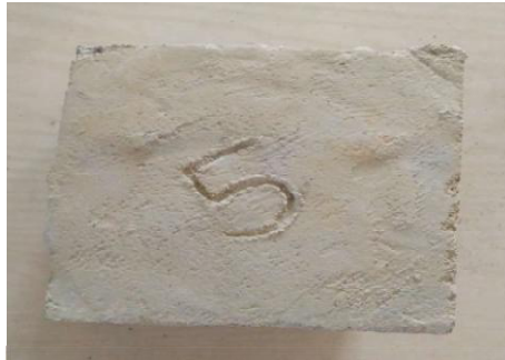
Fig. 5: Cube after curing
