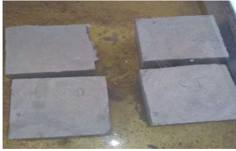
Fig. 4: Cubes put into tank for curing.
