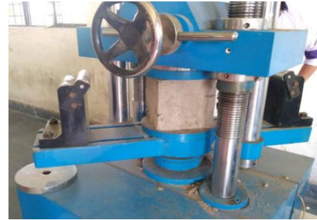
Fig.7: Testing the Compressive strength of the cubes.
